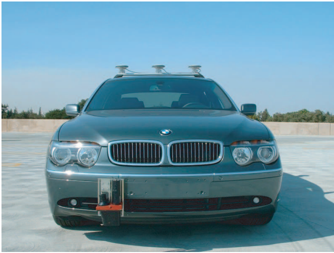
Figure 4. GPS ANTENNAS AND OPTICAL SENSOR MOUNTED ON EXPERIMENTAL VEHICLE
